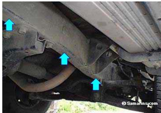
Korrosion am Kfz
